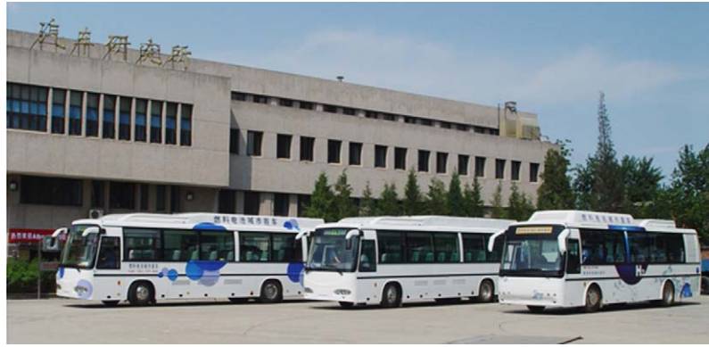
Fig. 1. The developed prototype of fuel cell city bus (from left to right that is testbed bus, practical bus A and practical bus B, respectively).
